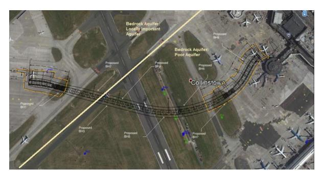
Figure 2-1: Orthophoto of the proposed tunnel route with the approximate aquifer boundary. The markings for proposed borehole locations are from the technical note: 'Review of Existing Geotechnical Information', however an updated borehole location plan can be found in 'Specification for Ground Investigation').
